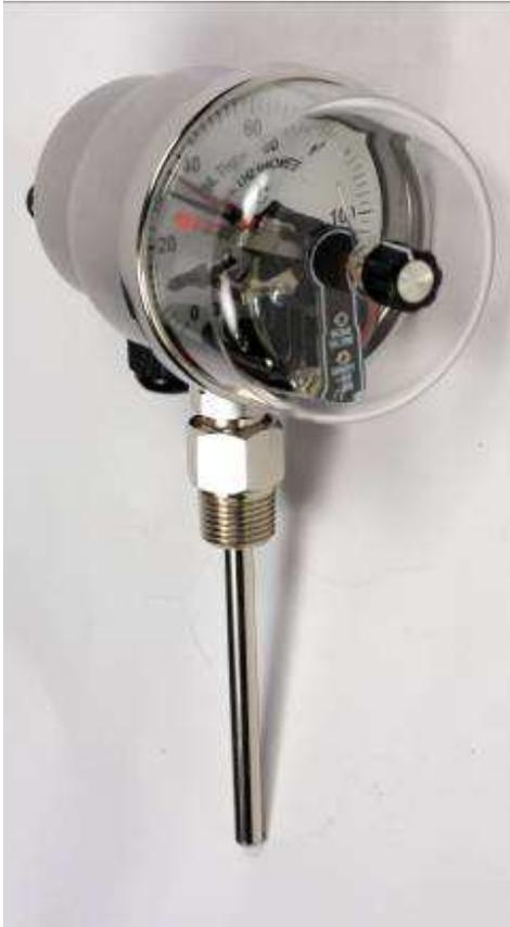
This instrument is designed to control temperature in oil filled TRANSFORMERS.
